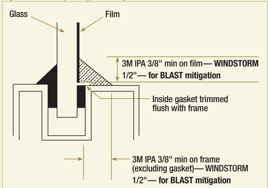
5. Carefully remove the two masking strips from the glass/frame immediately after tooling. Do not allow the excess adhesive to contact the film, frame or flooring surfaces. A light colored drop cloth is needed to protect the work area. **Be careful not to step on adhesive and transfer it to surrounding surfaces.**
